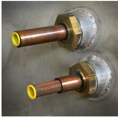
The lower fitting reveals the inner tube inside the outer wall.
